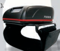
Secure, wrist-mount adjustable strap allowing access to rear panel functions
