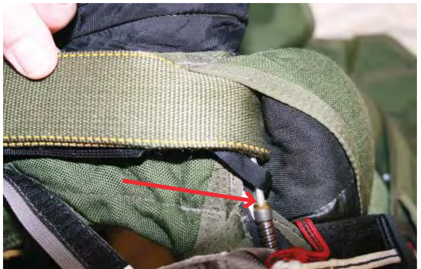
Figure 13. Cable is Fully Inserted
