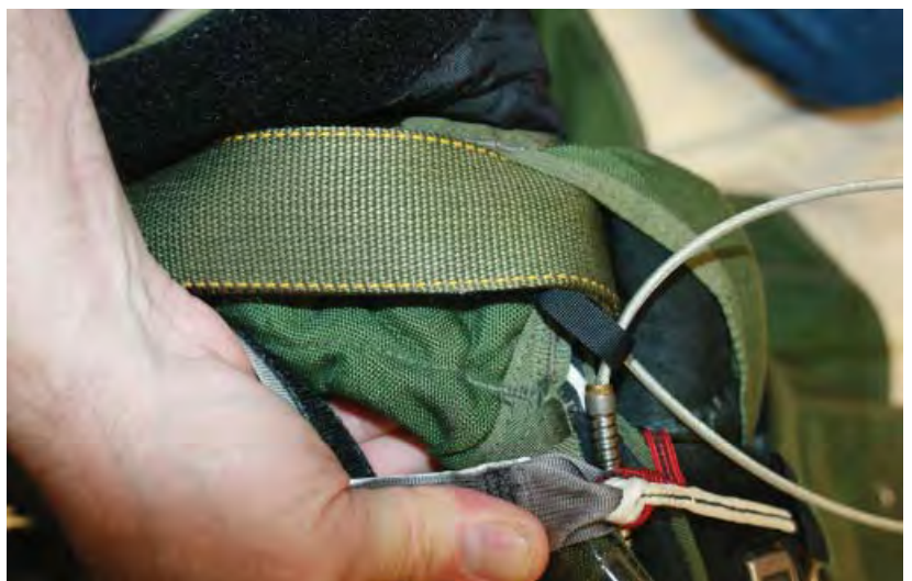
Figure 11. Cable Passes Only Through SCL
