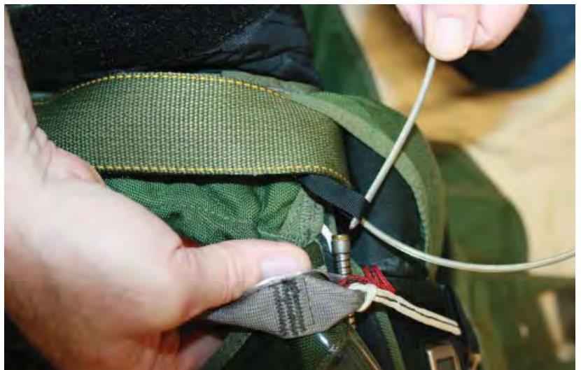
Figure 10. Insert Release Cable
