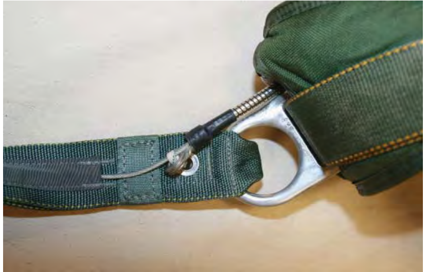
Figure 21. Riser Assembled Correctly
