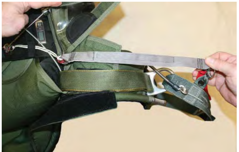
Figure 4. Remove RSL from Velcro
